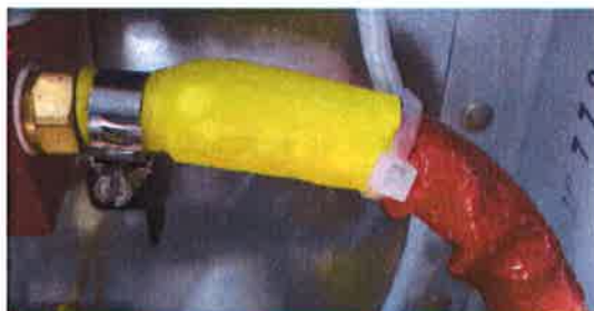
Fuel hose with Pyrojacket, hose clamp and Thermofit CGPT hose
