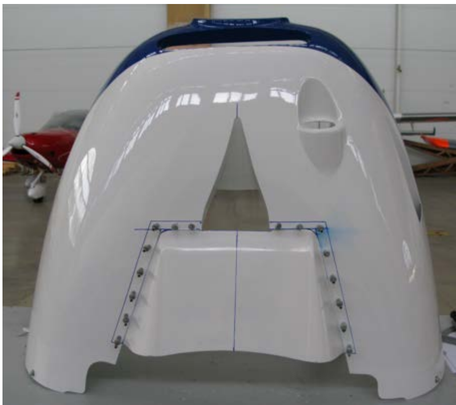
Figure 13: Fixing and gluing of the new cooling exhaust on the cowling
