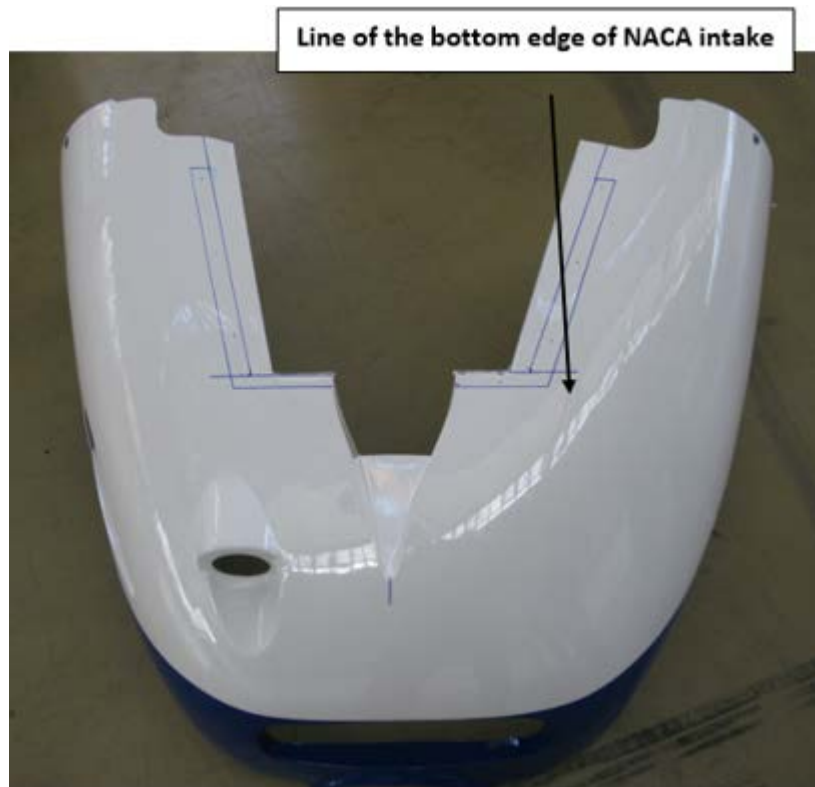
Figure 11: Helping lines for making cut-out in the engine lower cowling
