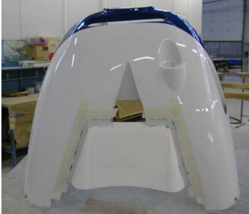
Figure 16: Sealed and grinded connection area
