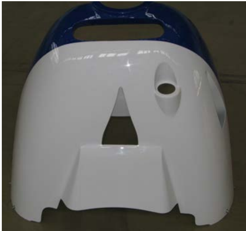
Figure 17: Completed lower cowling with the new air exhaust
