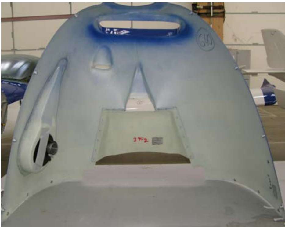
Figure 14: New cooling exhaust glued in the cowling – view of inner side
