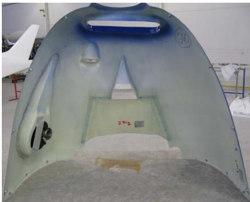
Figure 15: Laminated and grinded connection area with three layers of fabric
