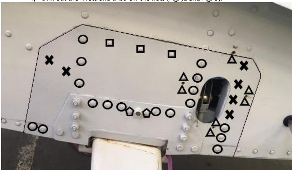
Fig. 2: Main gear attachment patch (left side)
