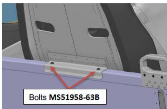
Locker SF0906N (upper) secured by two Bolts
