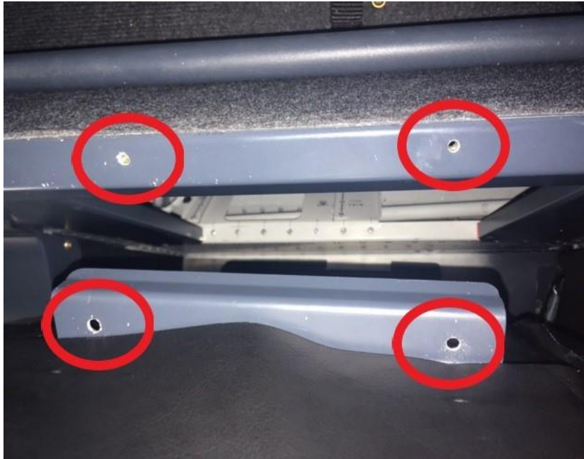
Fig. 10: Holes in the upper hook and backrest wall member
