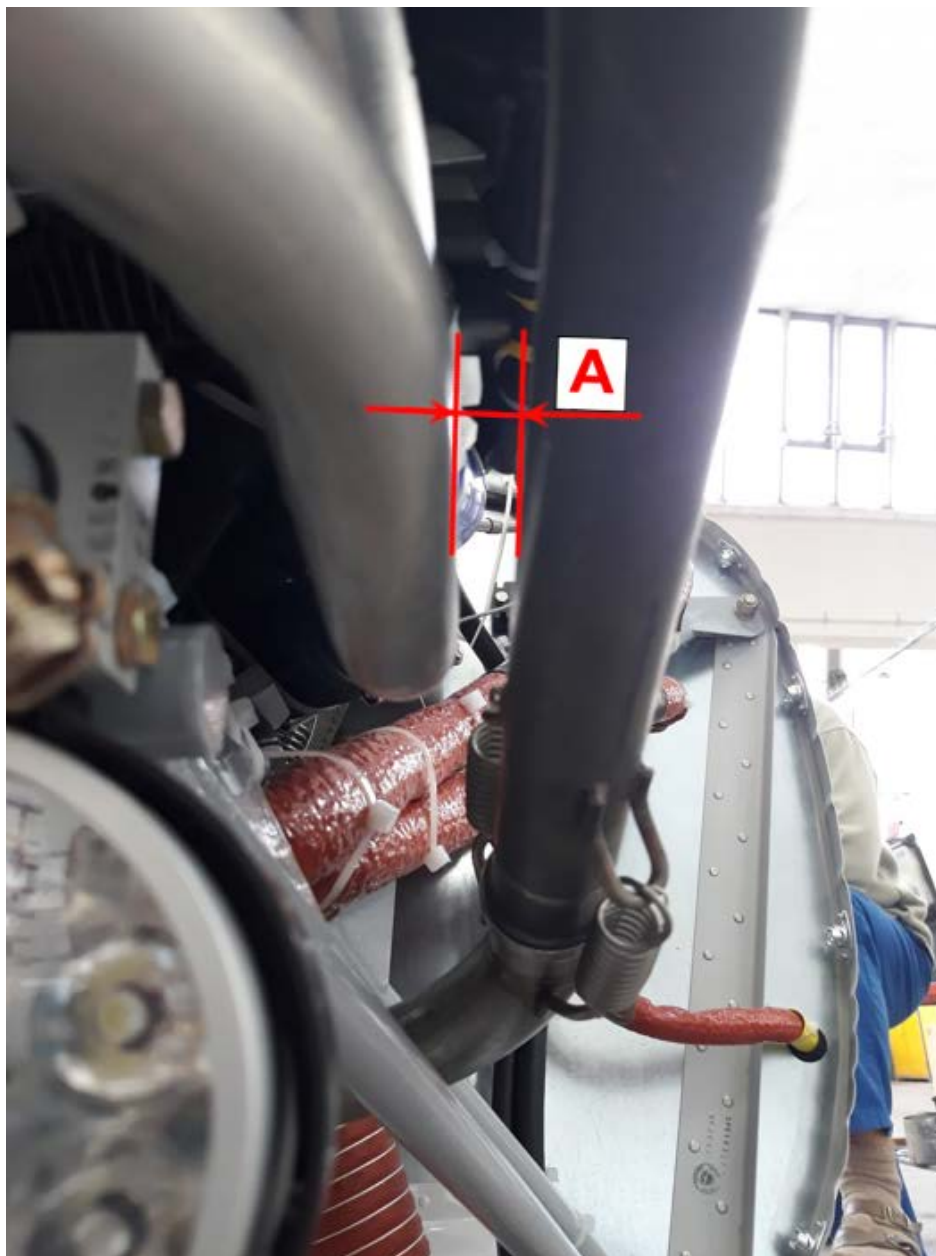
Figure 1: Distance between exhaust and coolant tube
