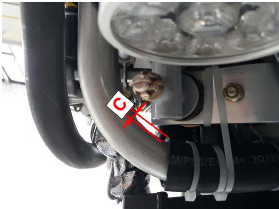
Figure 4: Distance between cooling tube and engine mount – right side – bottom view
