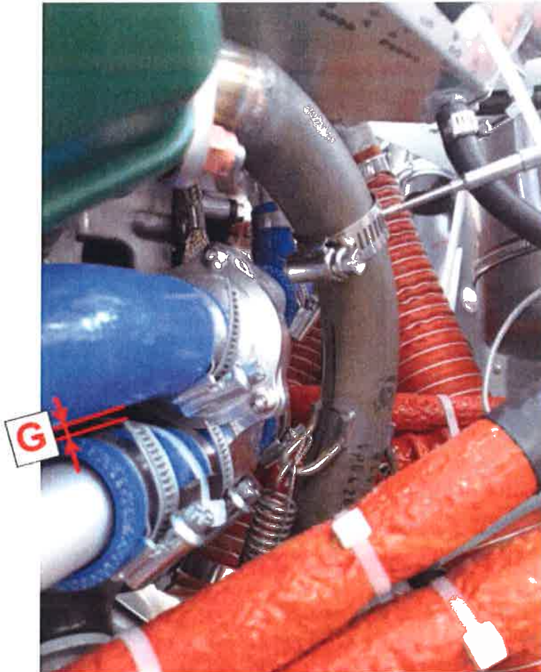
Figure 7: Distance between cooling tube and fixing stripe free ends
