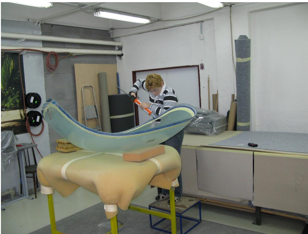
Fig. 30: Apply the sealant
