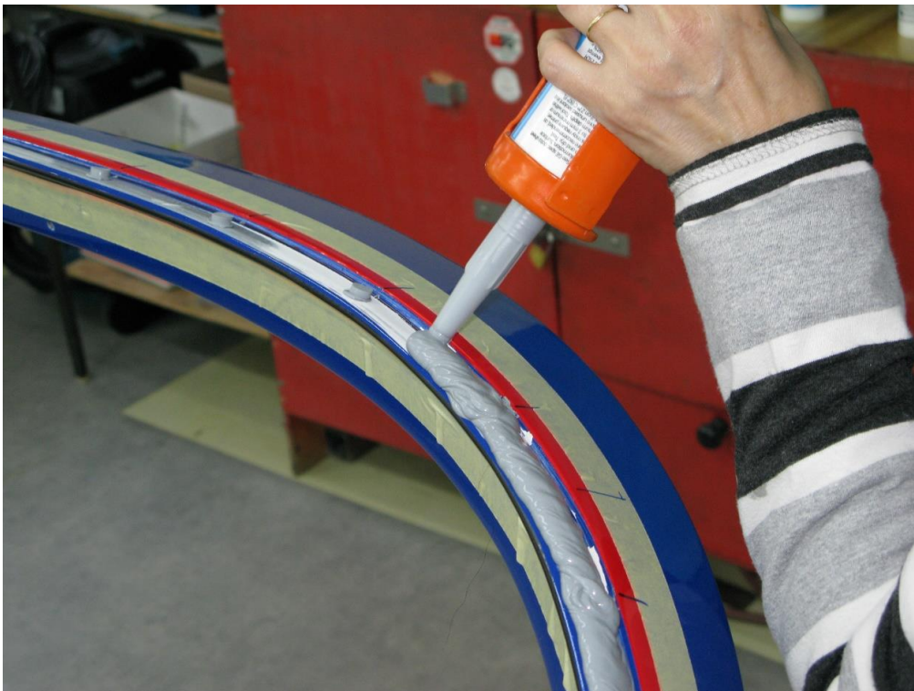
Fig. 32: Apply the sealant
