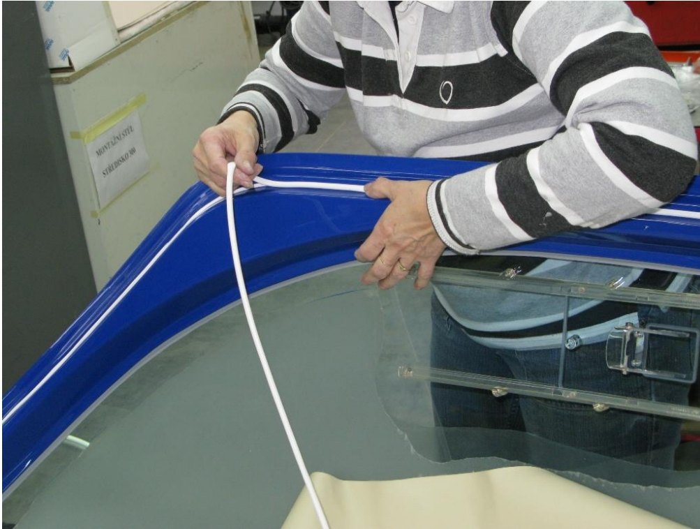
Fig. 55: Apply the sealant
