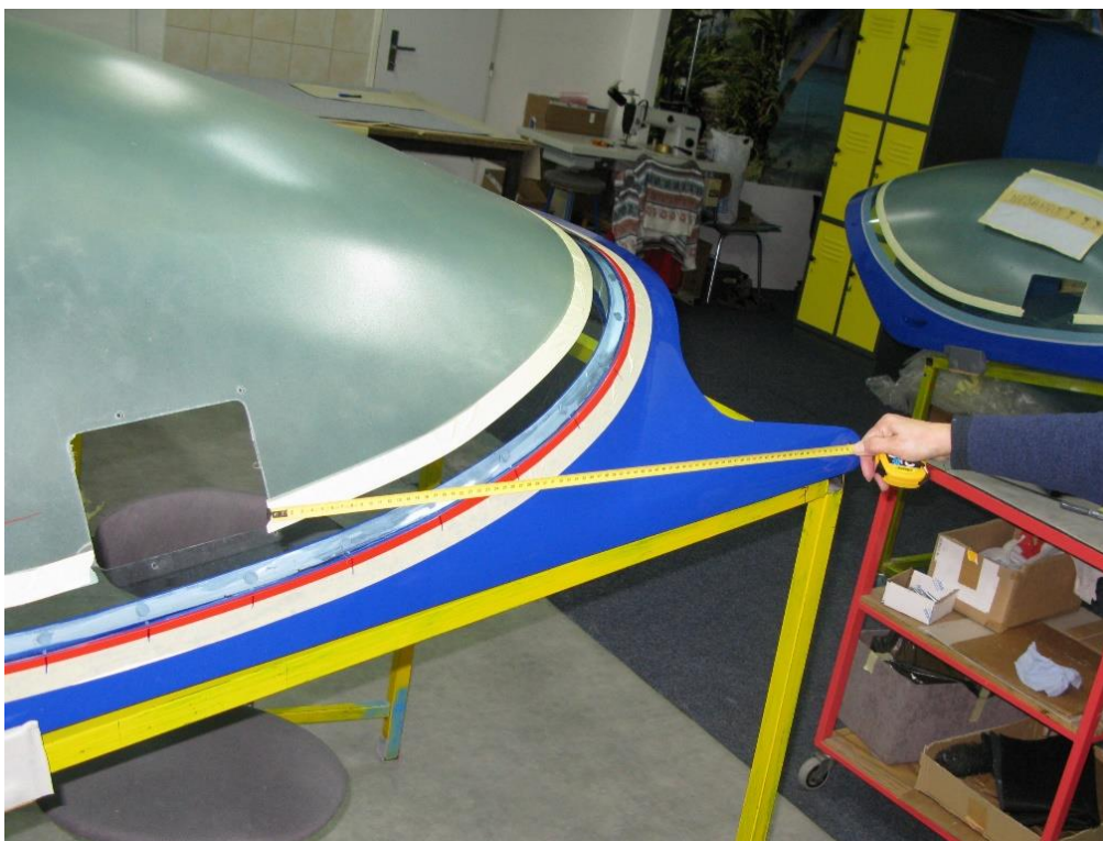
Fig. 17: Position the acrylic glass
