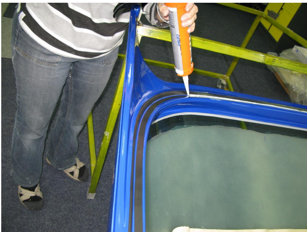
Fig. 54: Apply the sealant
