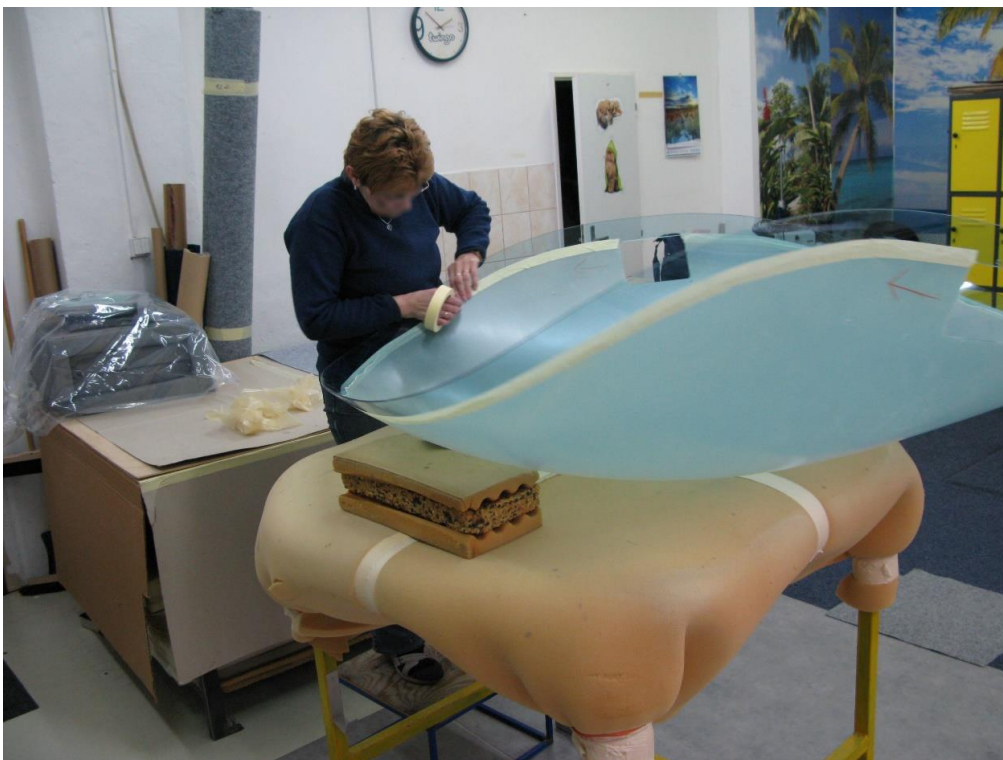
Fig. 16: Prepare inner protective foil
