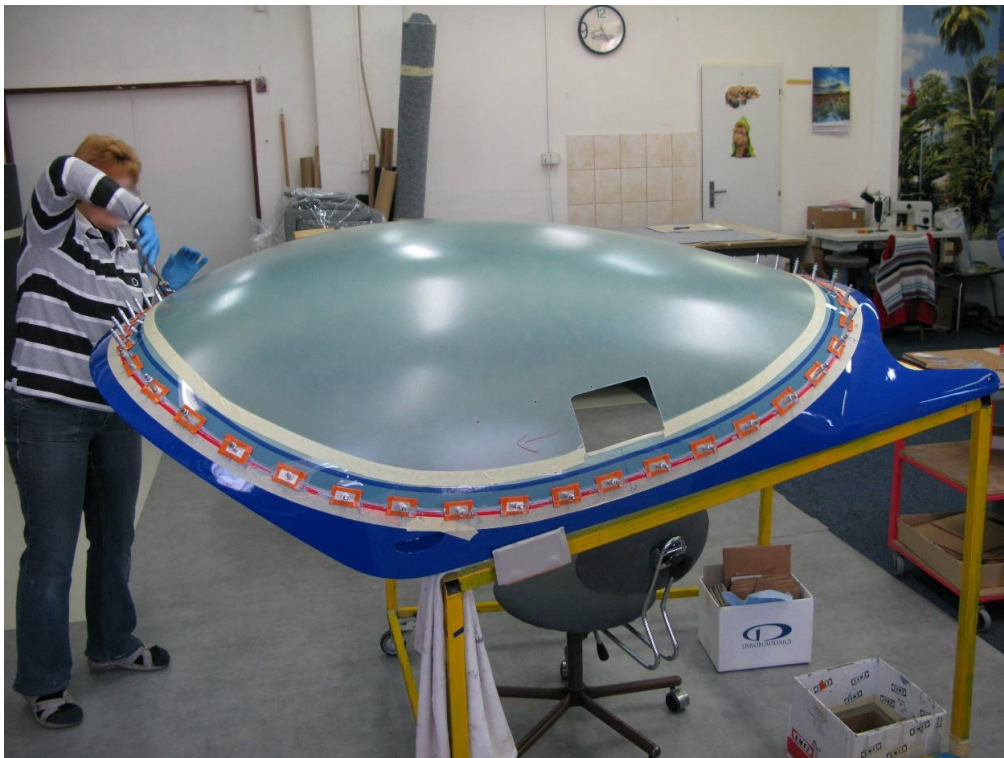
Fig. 34: Attach the acrylic glass
