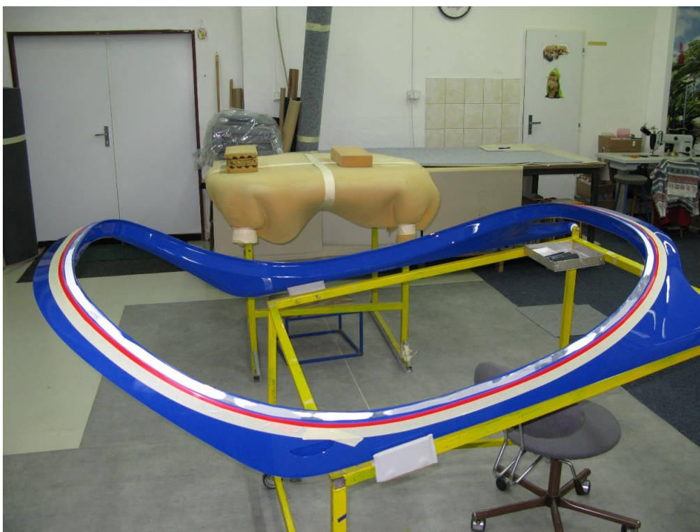
Fig. 2: Canopy frame without canopy glass
