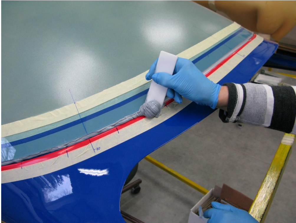
Fig. 33: Wipe off the excessive material
