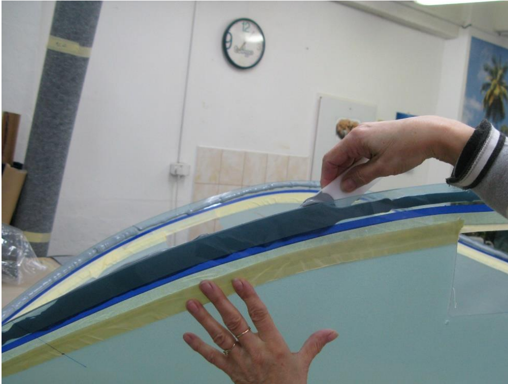
Fig. 31: Spread the sealant bead
