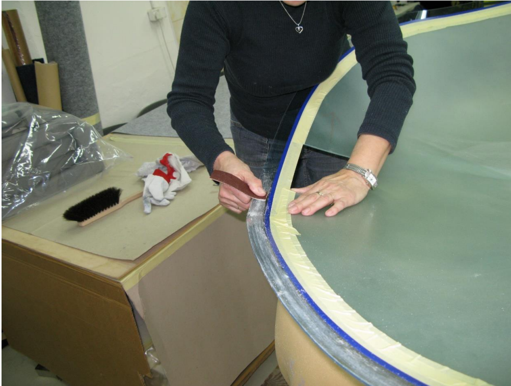
Fig. 29: Grinding the surface
