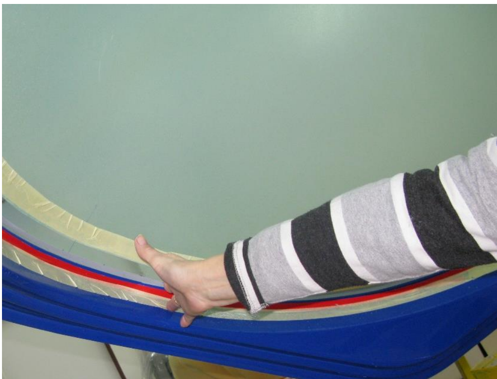
Fig. 37: Smooth out the field of sealant with finger
