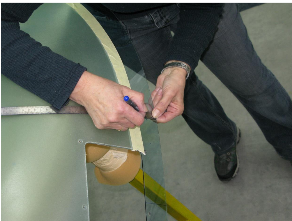
Fig. 26: Marking the line
