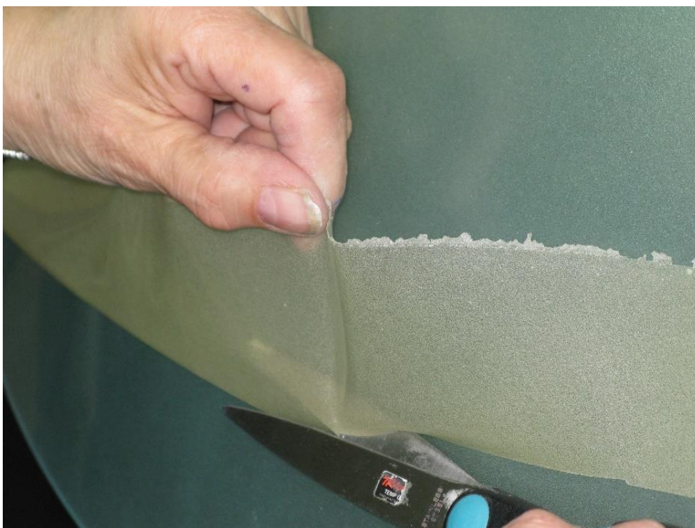
Fig. 14: Cutting the protective foil
