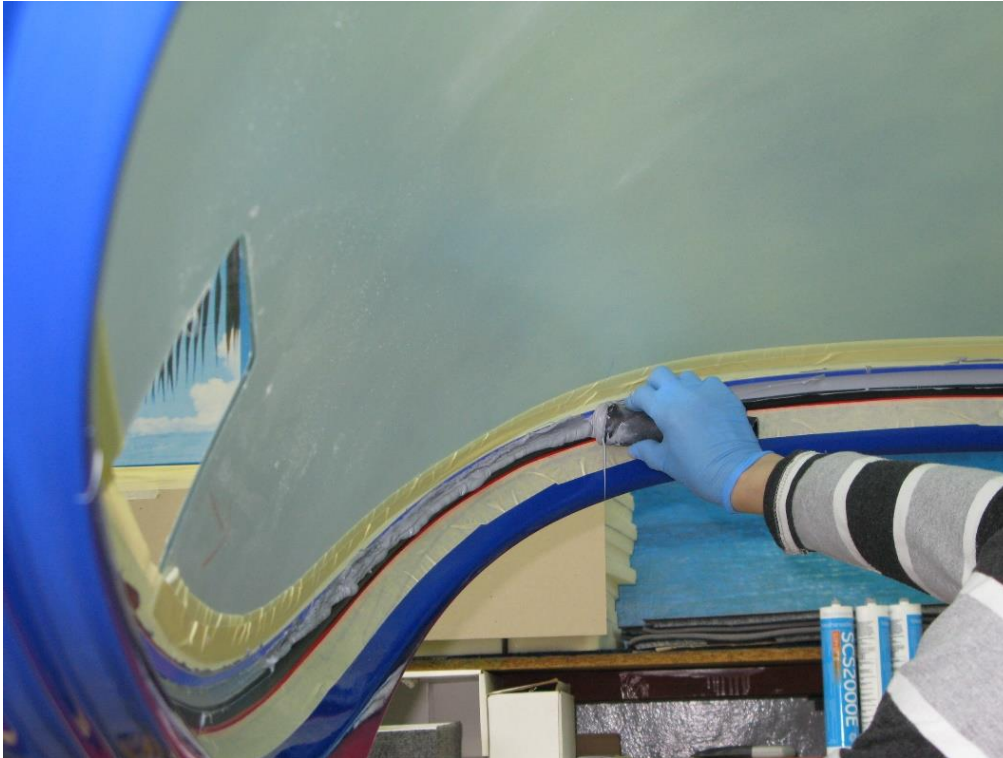
Fig. 35: Wipe off the excessive material
