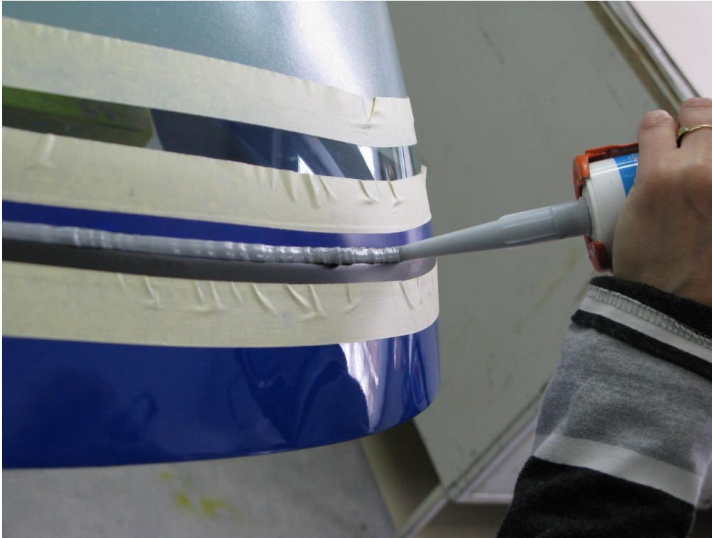
Fig. 47: Apply the sealant
