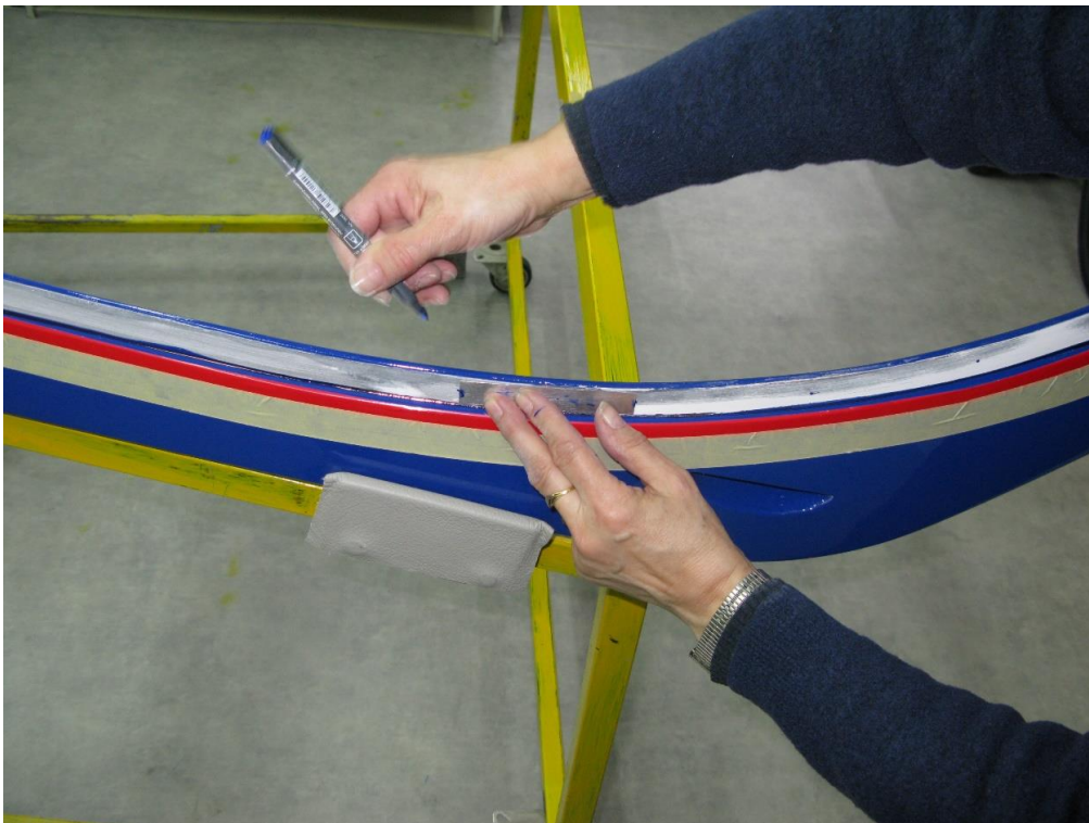
Fig. 6: Mark the surface line
