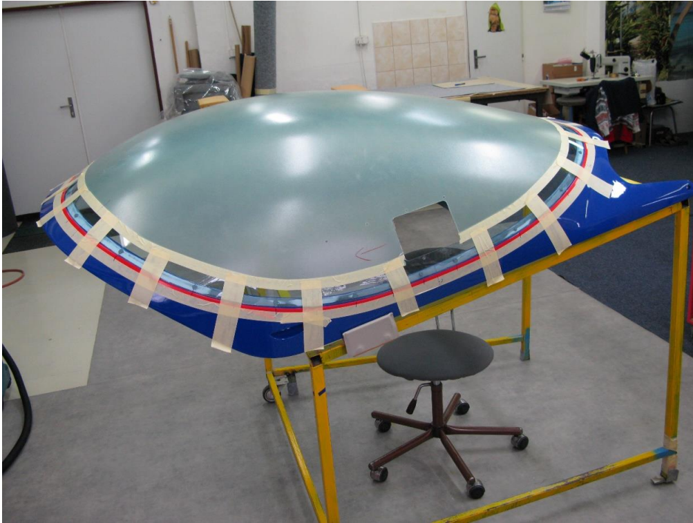
Fig. 23: Acrylic glass fixed with paper tape
