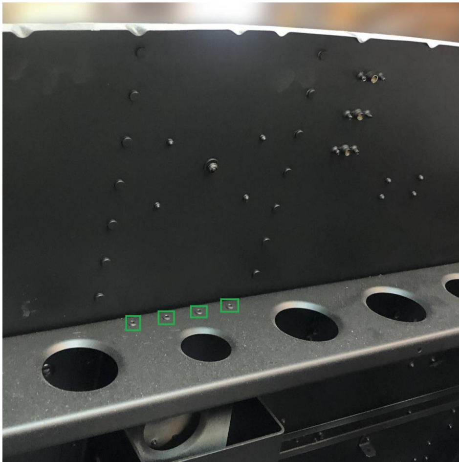
Fig. 7: Rivets from inner side of firewall
