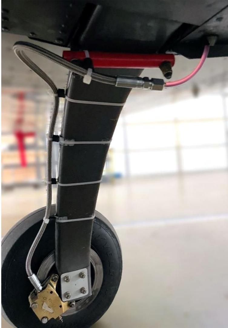
Fig. 4: Brake with metal brake hose
