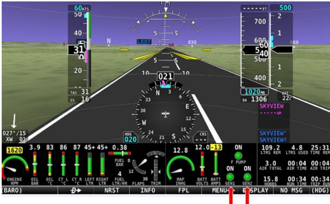
Fig. 6: Position of the GEN 1 and GEN 2 warning lights on the MFD screen
