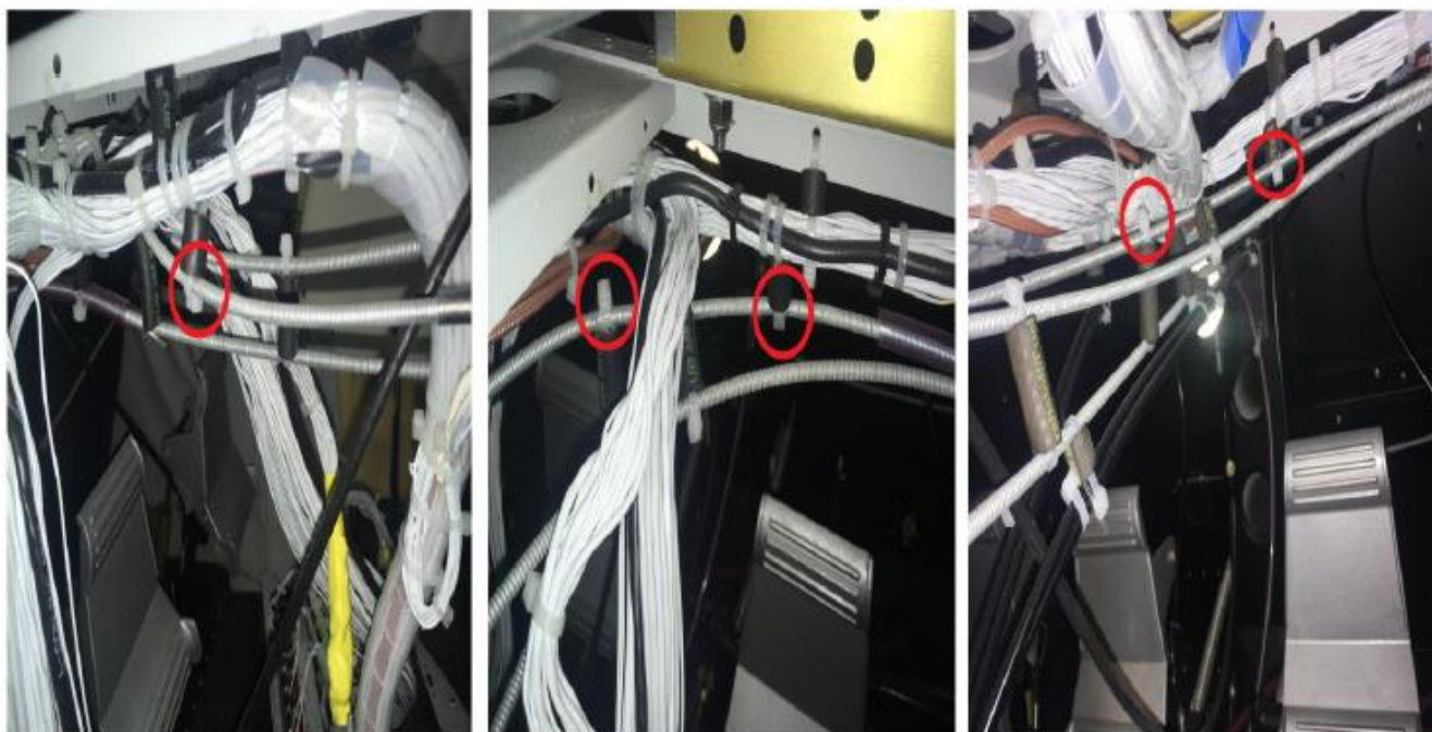
Fig. 8: Position of cable ties
