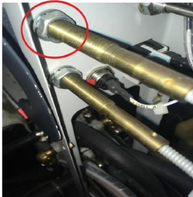
Fig. 20: Position cabin heater knob and nut
