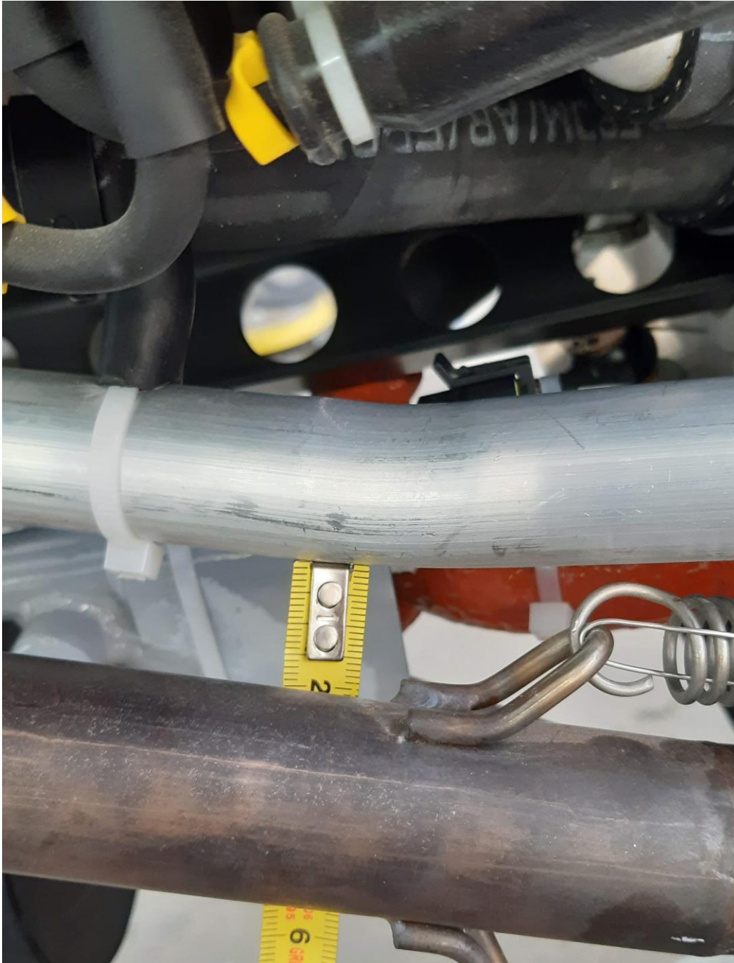
Fig. 20: Typical distance between left tube and left front exhaust.
