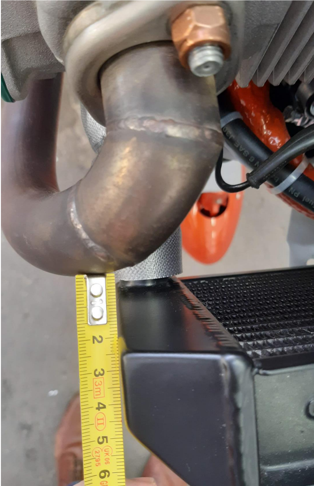
Fig. 17: Typical distance between right front exhaust and radiator
