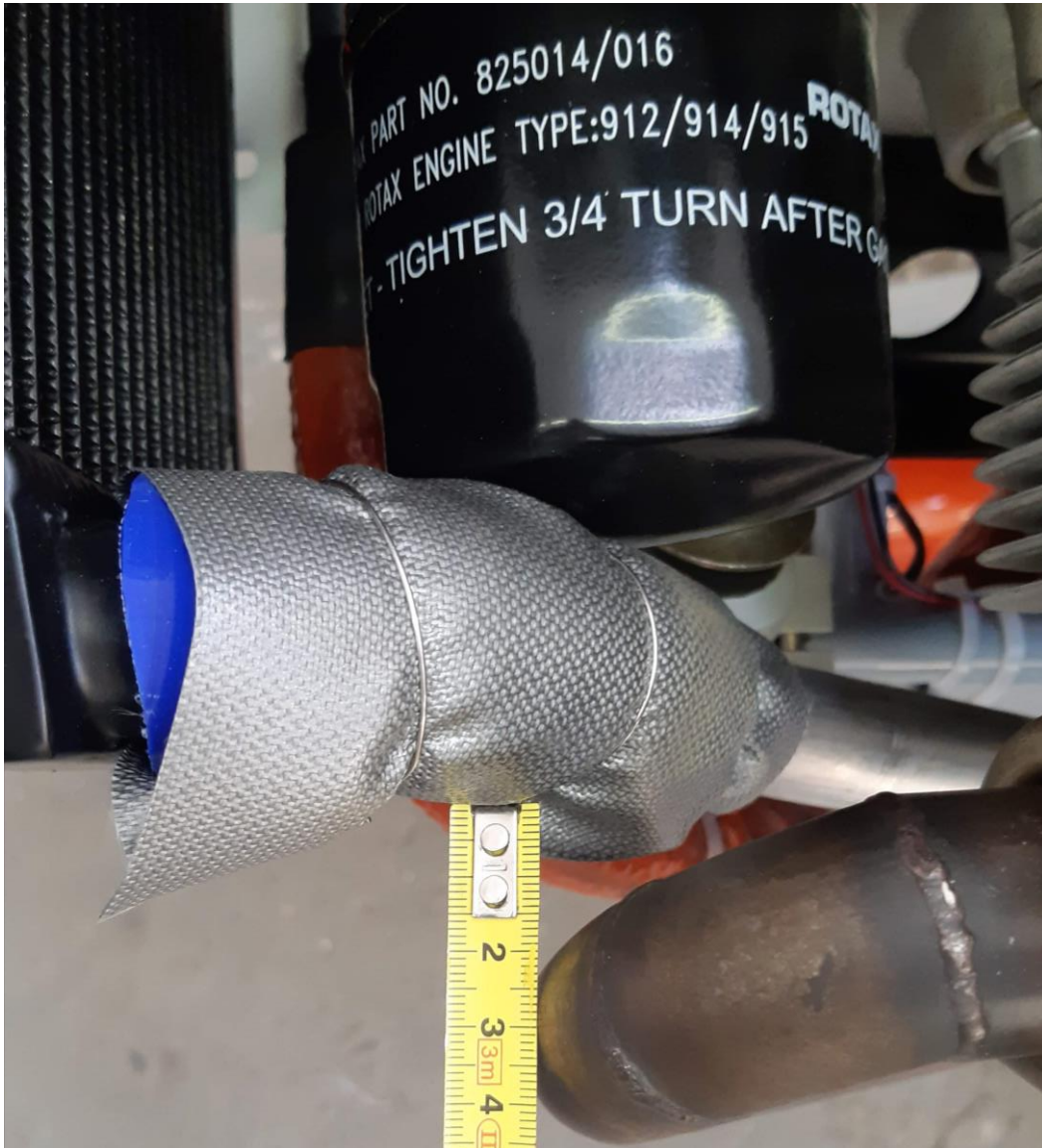
Fig. 19: Typical distance between left tube and left front exhaust.
